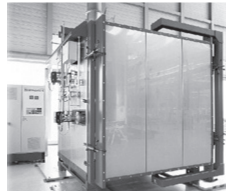
Chamber kiln for intermittent operation
