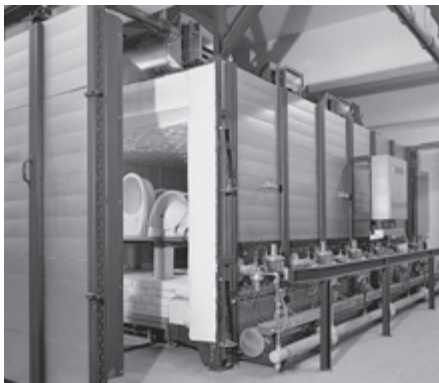
Ceramics kiln with temperature control via impulse system
