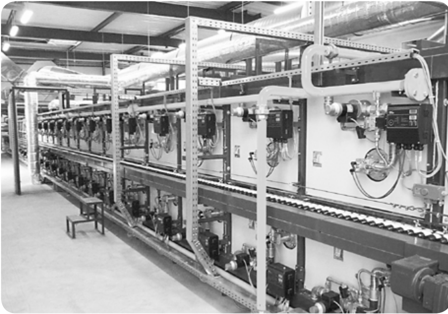
Roller hearth kiln in the ceramics industry
