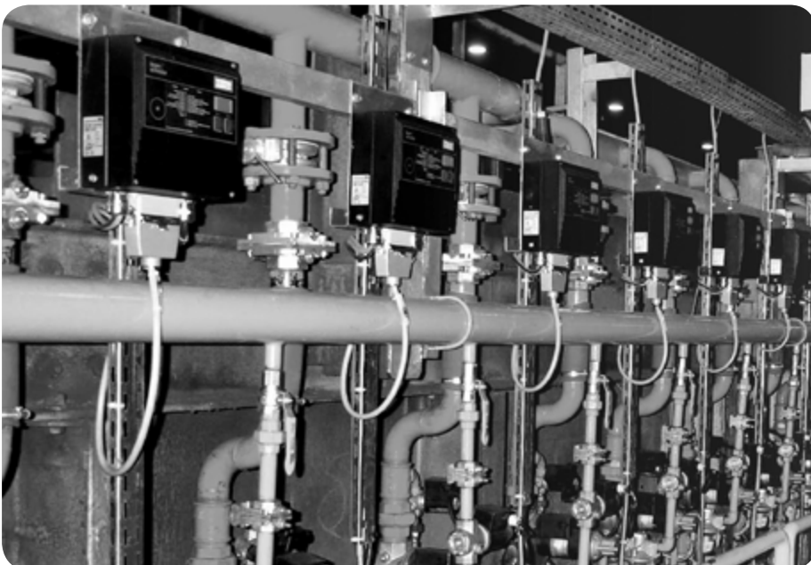
Hardening furnace with lots of industrial burners located side-by-side
